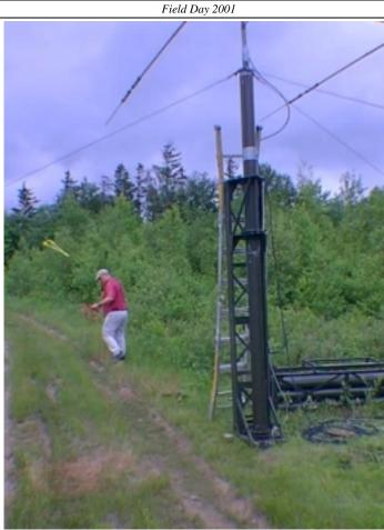
Fran (KM1Z) walking the 40 meter full wave delta loop antenna out away from the AB-577/GRC military surplus crankup tower with Fran's A3S tribander on board
