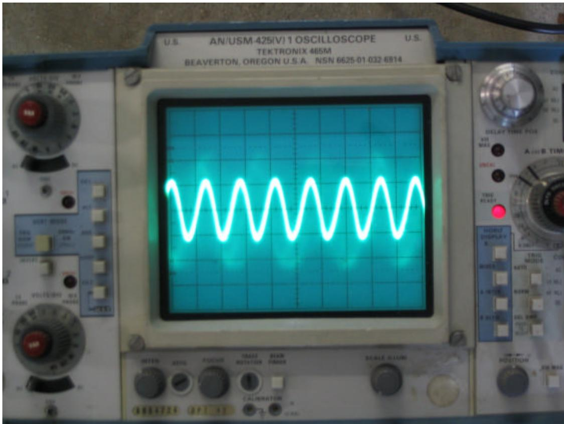
This is a picture of the sine wave output from our project board. The vertical scale is 5mv/division and the horizontal scale is 1 ms/division. As displayed, the output is 12.5mv PP at approximately is 714 Hz (5 complete cycles in 7 ms).
