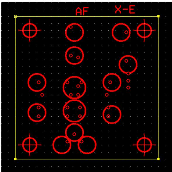
You will notice, right away, that all of the component outlines, ID's, and ground connections have disappeared. The very small circles are component connections for lead # 1 of the various components. For our purposes, ignore these. All that remains are the islands and the mounting hole circles. Cut the pattern along the board edges in the printout to produce the 2" X 2" cutting template.
