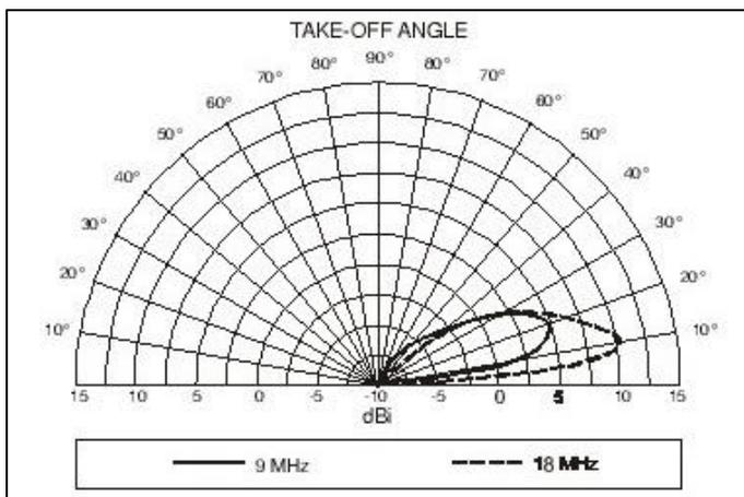
Fig. 3 Vertical pattern for sloping vee with 30 degree apex angle.
