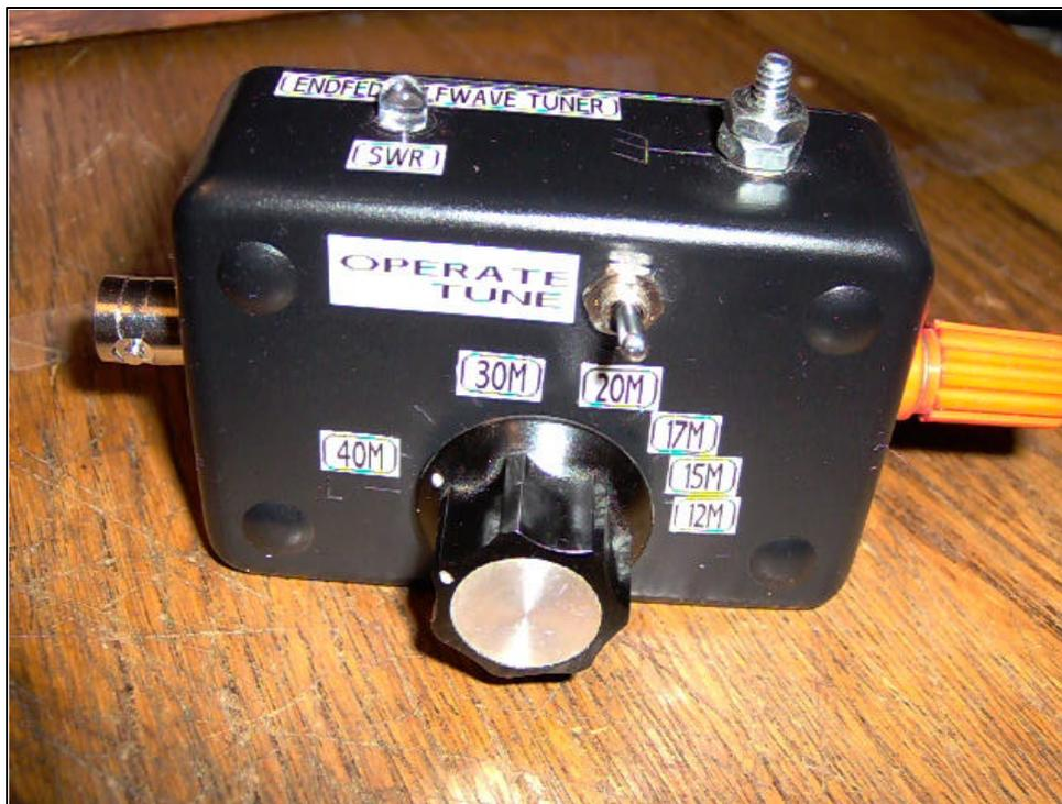
With the SWR bridge switch in the operate position, adjust the capacitor for maximum receiver signal or noise, then put the switch in the tune position, key the transmitter and watch the LED as you fine tune the antenna to get the LED to go out. Once the LED is off, put the switch back into the operate position, and you are ready to transmit. Refer to the schematic to help explain how to build the tuner. It is a very simple circuit to reproduce. Have fun building, and
