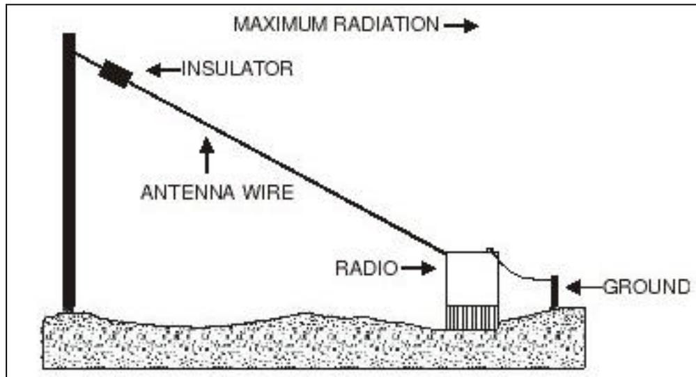
Fig. 6 Sloping wire antenna.
