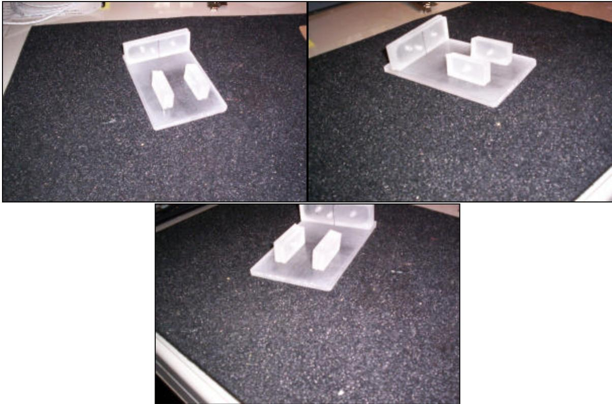
All components are cut. The holes for the screws having been centered and drilled. I sanded them to insure proper fit and epoxied them in place several times actually. I couldn't seem to get them aligned as I desired.
