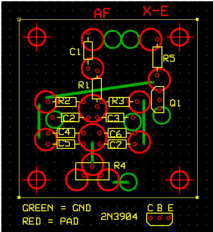
Dimensions are in real values. In other words, if I place a 1/4" diameter circle on the drawing surface, it will be 1/4" in diameter on the printed copy. A 1/4 watt resistor is approximately 0.1" wide and approximately 0.4" long. On the printed copy, it will have those dimensions.
