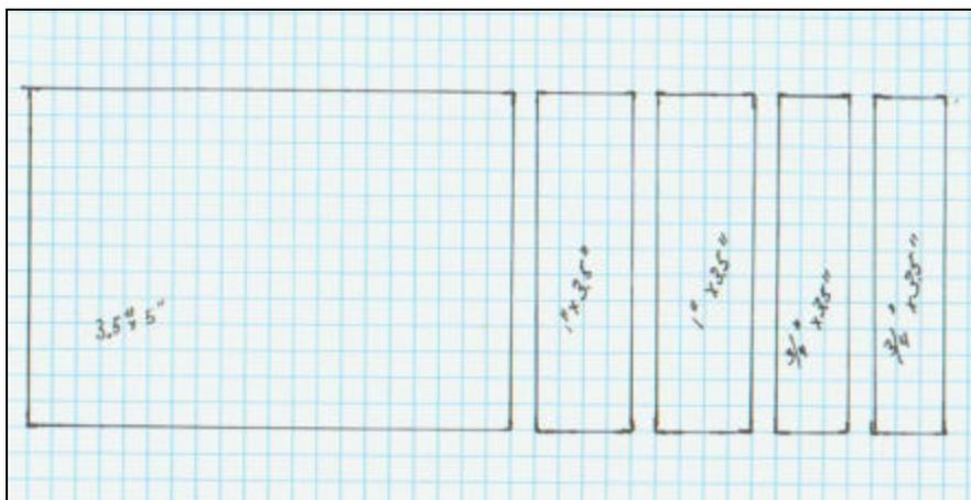
Using only a common hack saw to cut the 1/4" plexiglass. I cut the base the same size as Bill's 3.5" X 5". Now where Bill used some 3/4" X 3/4" wood stock for the Back Plate I cut 2ea 1" X 3.5" strips these will be epoxied together to form the needed Back Plate. The 3/4" X 3.5" strips will also be epoxied together then cut in half to form "DOT" and "DASH" adjustment screws plates
