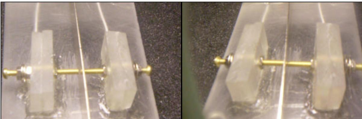
The Back Plate is shown here. Notice connecting wires from the Adjust Srews are run under the Base plate.
