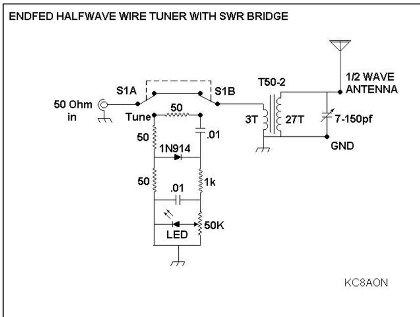
The 50 ohm side goes to the 3 turn link, and the hi Z antenna connects to the ungrounded end of the 27 turn winding. The variable capacitor connects across the antenna side from the ground to the antenna terminal. The variable capacitor in this tiny tuner was salvaged from an old AM broadcast band transistor radio that I picked up at a flea market for 50 cents ! If you see these old radios cheap at flea markets, grab them - the vari caps are valuable !
