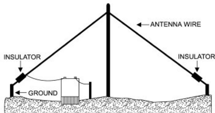
The center support is about 50 feet high. Terminate the end away from the transmitter with a 600 ohm resistor between the antenna wire and a ground rod. For frequencies below 12 MHz, point the terminated end in the direction to be favored. For frequencies above 12 MHz, the favored directions will be about 10 degrees off either side of the wire, toward the terminated end. This one makes a great field antenna for medium to long range contacts.
