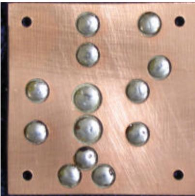
In this picture, the PC board has been cleaned and the islands tinned. An ohmmeter has been used to verify that the islands are isolated from the copper ground plane.
